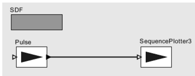
FIGURE 9.6. A model that plots the values of a signal. 256 iterations must be executed to plot the entire signal.
